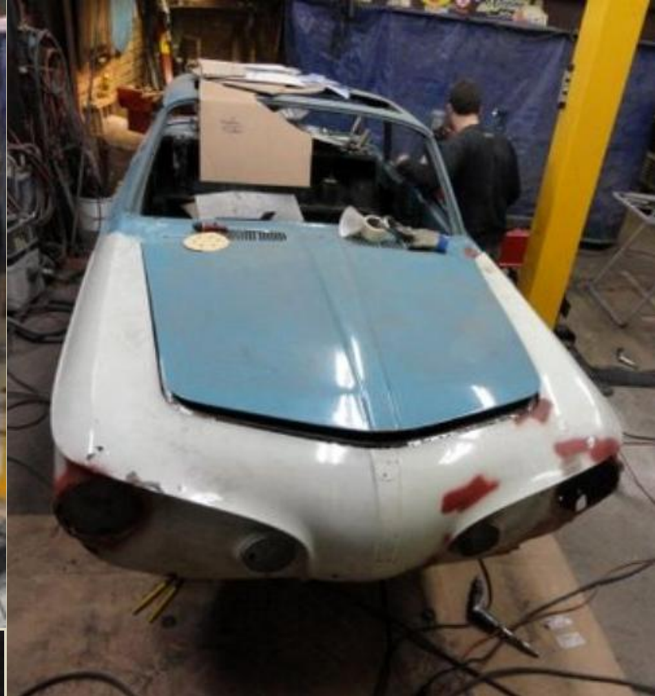
Now the front skin has been welded into place. The original front hood, fresh-air vents, & inner front compartment metal was retained. Next step is to complete the left side rocker.
