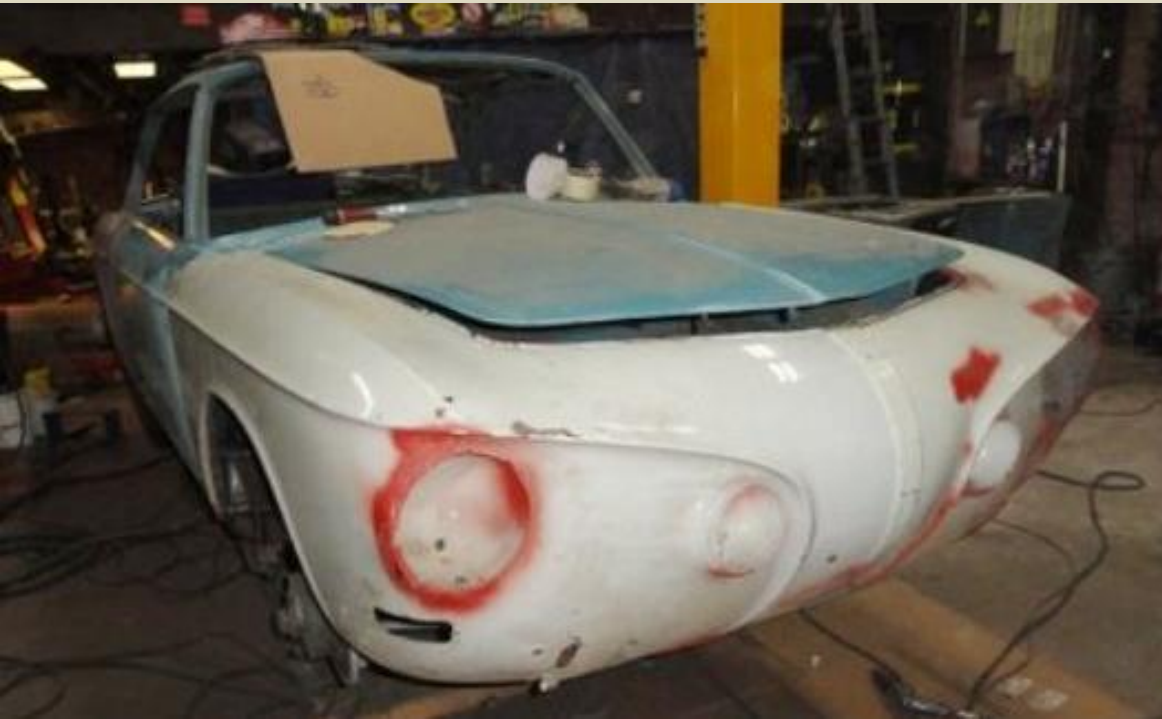
Now the front skin has been welded into place. The original front hood, fresh-air vents, & inner front compartment metal was retained. Next step is to complete the left side rocker.
