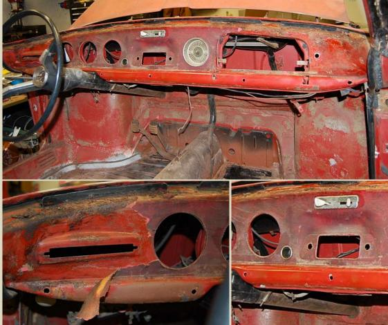
Once Thom made it to disassembling the instrument panel he discovered the previous owner had glued a vinyl covering over the Ruby Red dash. Another unpleasant discovery was the rust along the top-left edge underneath the upper dash pad and the mounting bolts (cast into the dash pad foam) had completely disintegrated.
