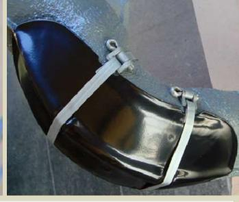
Position the shield & straps loosely. Originally VW had the clamps on the inboard sides. The strap wraps around the heat exchanger once, threads through the rectangular hole on the clamp, then wraps around a second time and threads through the cotter key. Pull in the slack and then trim off some of the excess strapping. Then tighten the key with a screwdriver a half-turn at a time, stopping to adjust the strap and reposition as necessary as you go. Turned out very nice!
