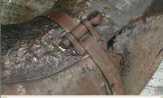
I did some research on substitutes for the coating and settled on Lizard Skin (www.lizardskin.com) ceramic insulation. It's not cheap but it has properties that make it a good choice for the job: good heat & sound insulation, withstands temperatures to 500°F, water based & non-toxic. I applied it with a brush over ISP West's ceramic coating, recreating the original texture, and then gave it several coats of engine enamel.
