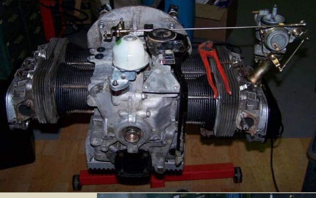
I also had all of the non-chrome metal galvanized parts including the door regulators, window screws, & bolts. Black powder-coating was applied to the engine sheet metal and spare tire carrier. The fuel tank was rusty so it was de-rusted first and then coated with a plastic solution inside. The engine was rebuilt & reassembled. lt's nice to see these old parts new once again!"
