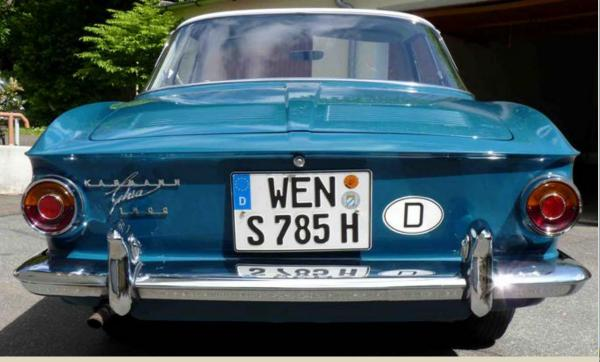
The 1962 features the KG script on the left-rear panel vs the right decklid in the later years. And the 1500 rear script has no tabs at the ends, unique from the tabbed 1500 version fitted to the 1963-65 models.
