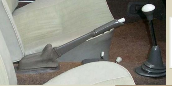
Pedro uses a special Adhesion Promoter clear primer that sticks to the rubber and acts as a primer, allowing the Anthracite paint to be applied better, dry faster, and not crack when the rubber boot is bent during the installation.
