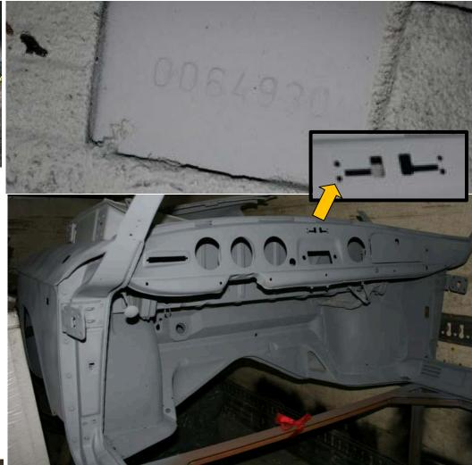
separate lever design & four mounting holes. So the two-piece design didn't end exactly when Karmann claimed the model year changed over.
